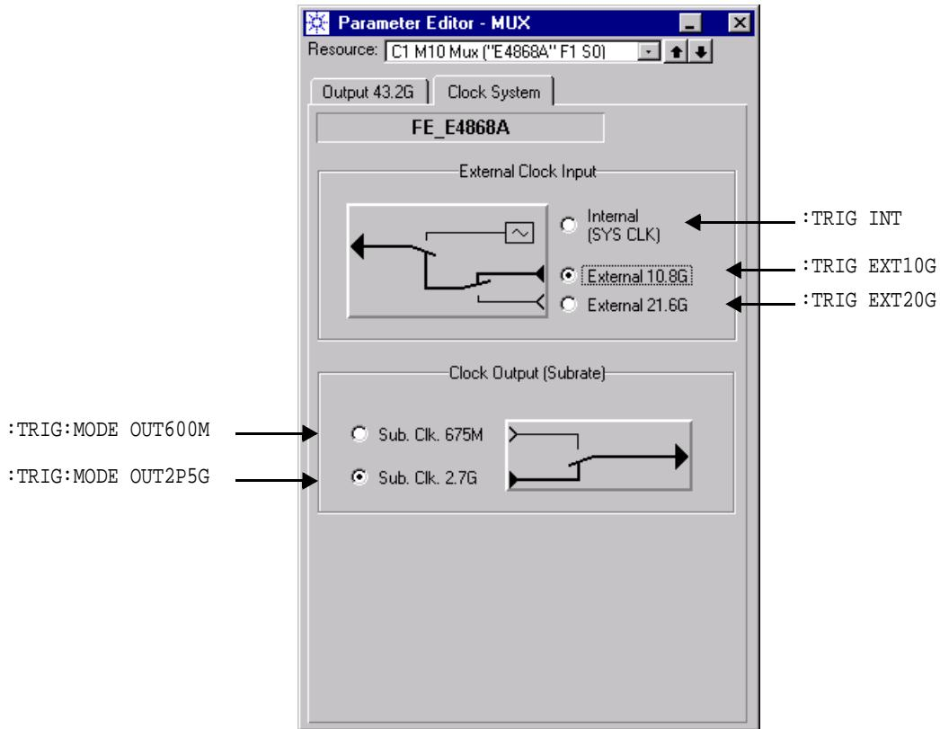
The following figure shows the clock system commands in the ParBERT user interface for a DeMUX module:
